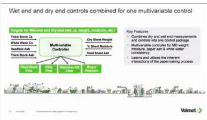
Fig. 7: Valmet – Wet and Dry End Controls.
