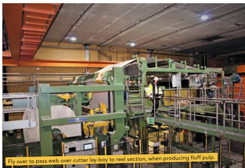
Winder/unwinder section with new parent reel feeding and empty spool lifting.
